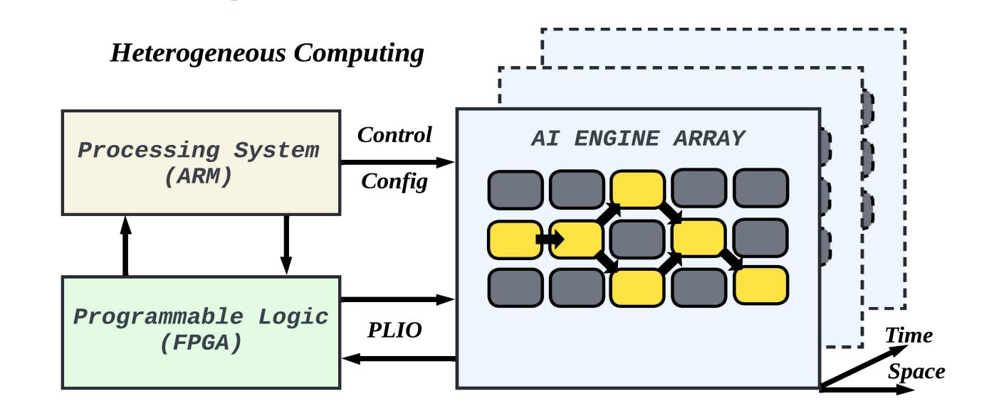
FPGA is a fine-grained reconfigurable architecture capable of efficiently performing data preprocessing tasks and implementing specialized hierarchical caches to hide memory access latency.
